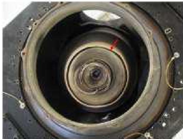
Photo No. 38. Exhaust case inner wall and PT input shaft housing
